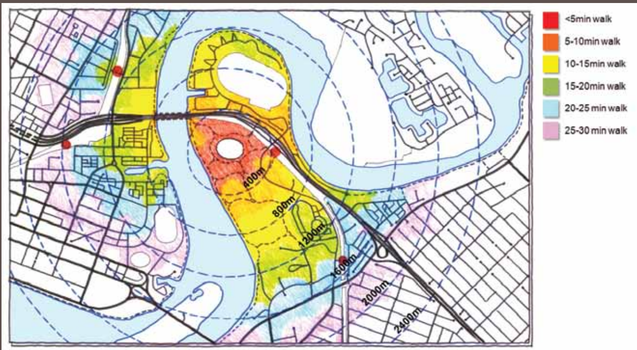
Ped-Shed Analysis – Bridge Not Included
